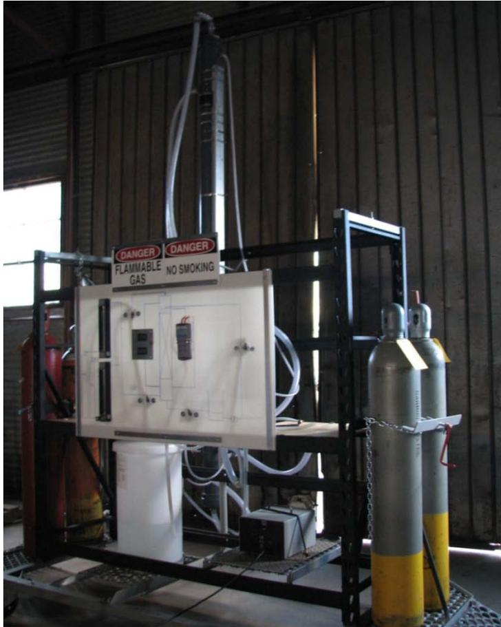
Figure 9.7: Experimental biogas purification set-up.
