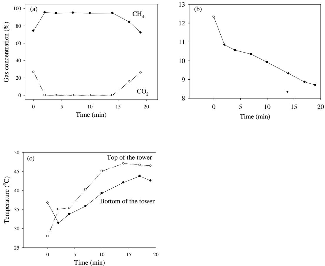
Figure 9.10: Biogas purification results with 20% MEA
