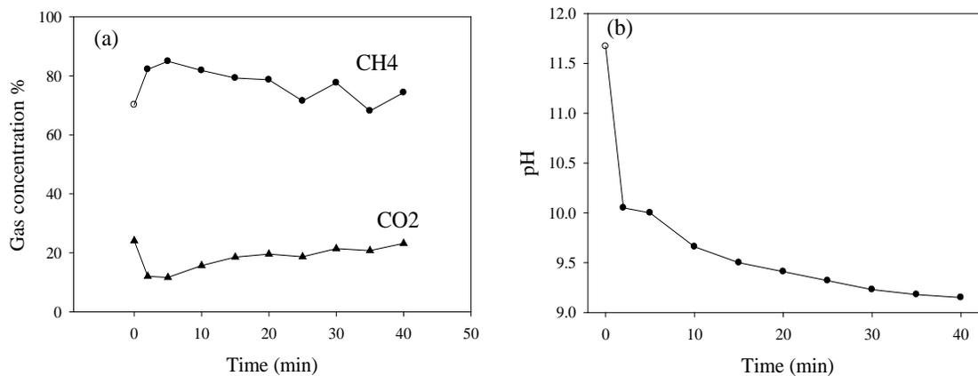
Figure 9.9: Biogas purification results with 40% MDEA.
