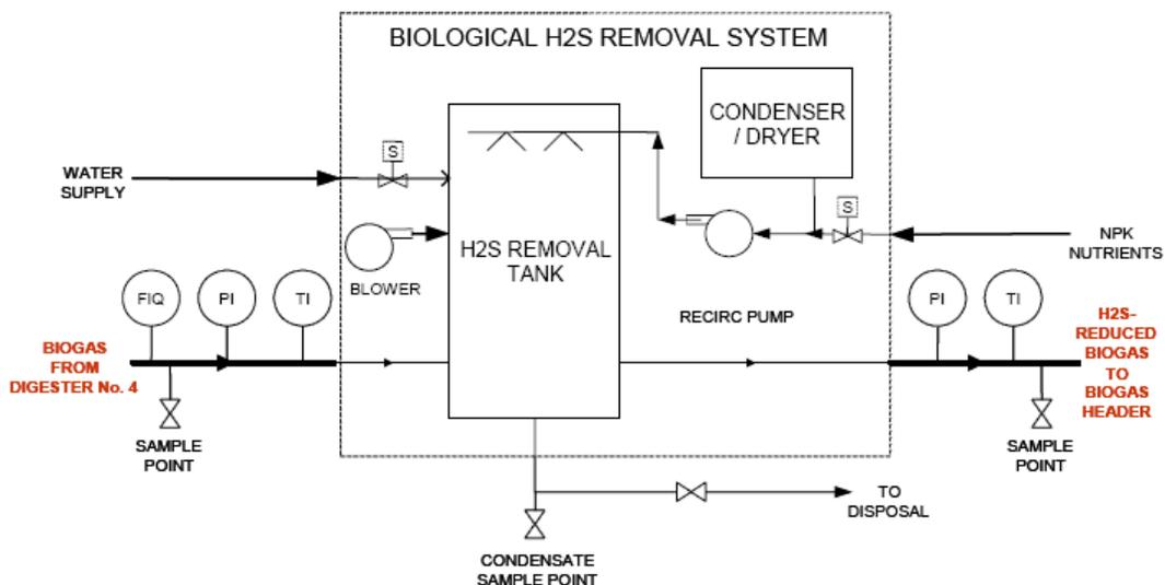
Figure 9.5: Biological H<sub>2</sub>S removal system (Soroushian et al., 2006)
