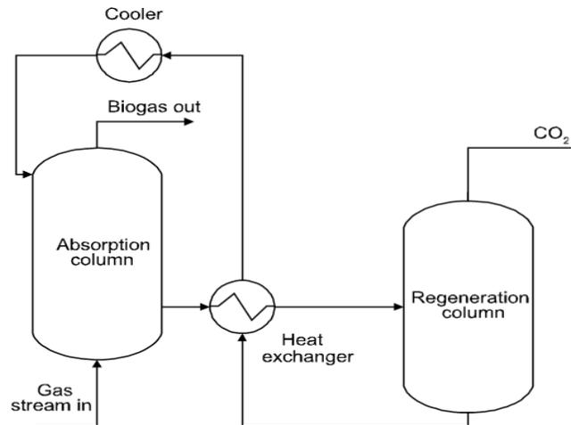
Figure 9.2: Flow chart of chemical absorption process
