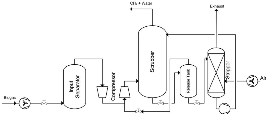
Figure 9.1: Flow chart of water scrubbing technology
