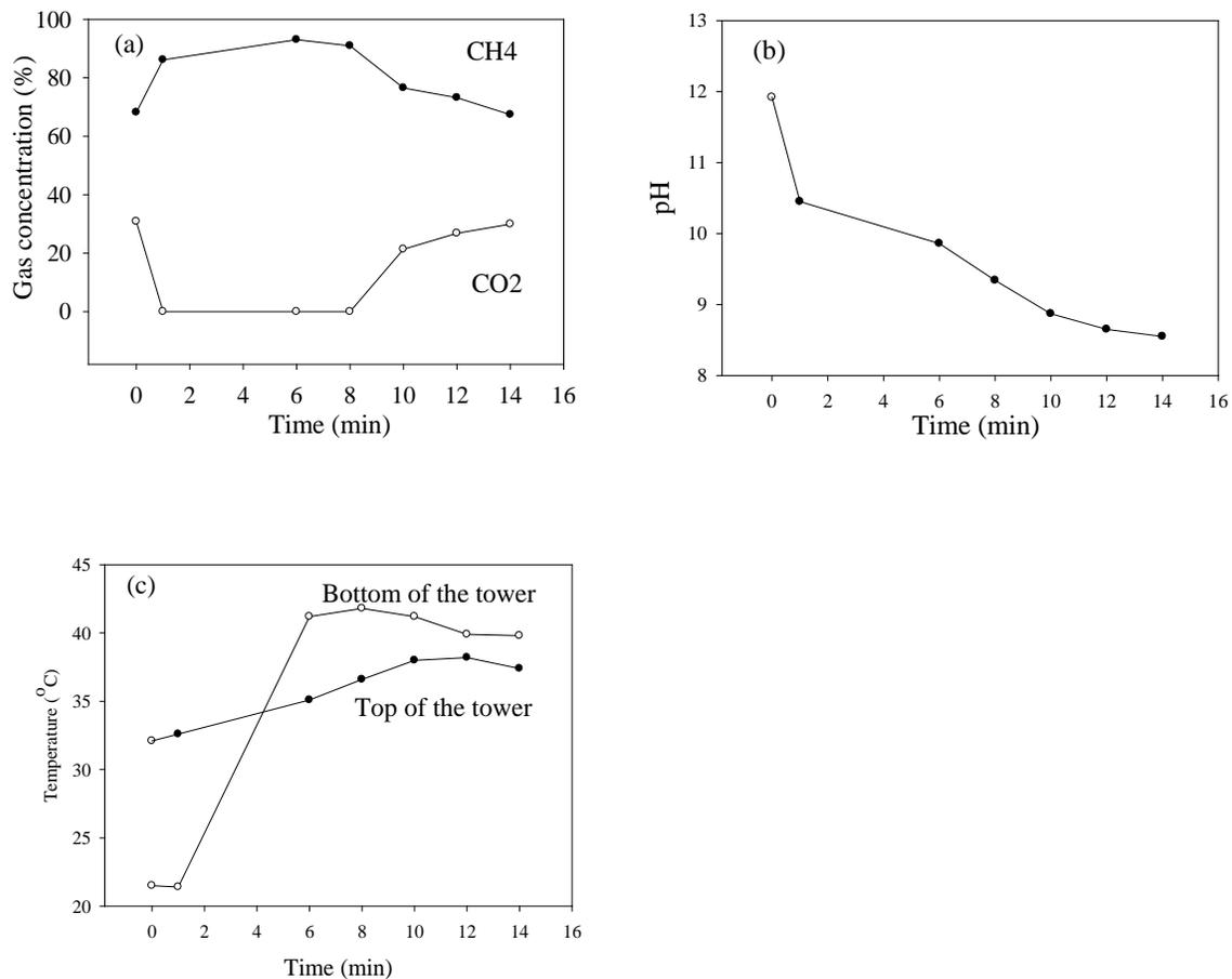
Figure 9.11: Biogas purification results with 10% MEA
