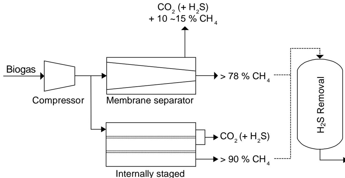
Figure 9.4: Flow chart of membrane biogas purification process
